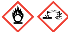
Flame over circle Corrosion
